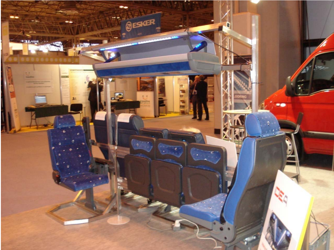
(Eurobus Idea): The Idea lightweight suspended system, displayed alongside Rescroft's new tip-up seats for side mounting into urban city buses and a swivel and tip-up seat for wheelchair accessibility
